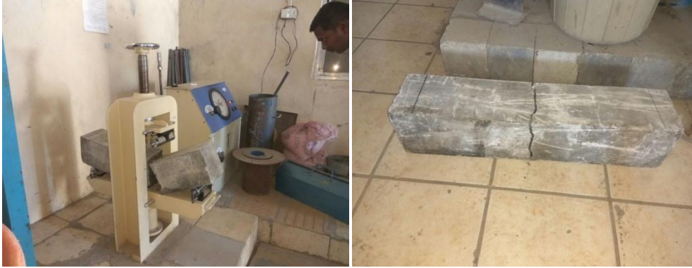
Fig-3: Crack Pattern For Usual PQC Beam
