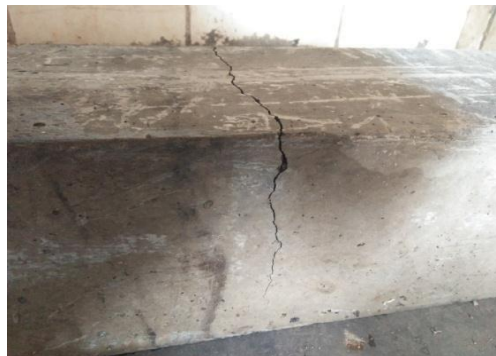
Fig-5: Crack Pattern For Biaxial Geo-grid Beam
